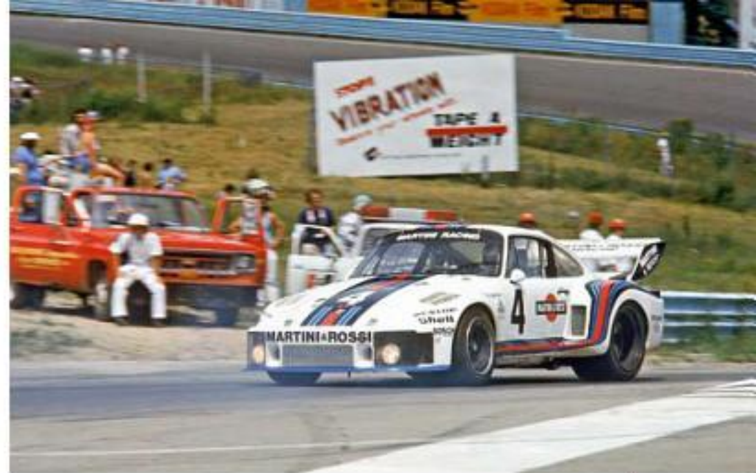
The Stommelen/Schurti 935 at Watkins Glen. Note the wheel covers, fitted halfway through the season to enhance brake cooling.
