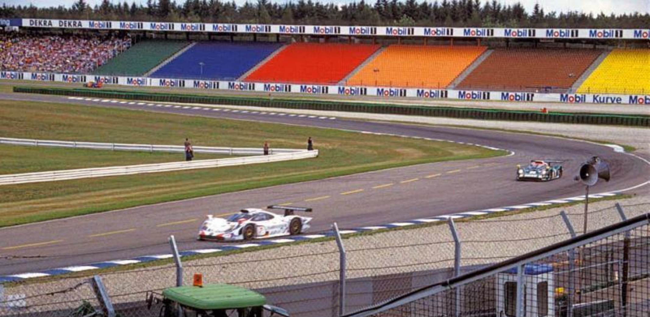
FIA GT action from Hockenheim with the works GT1/98 (chassis 003) of Yannick Dalmas and Allan McNish being chased by a Zakspeed car (chassis 004). The factory GT1s used Michelin tyres, while Zakspeed found its Pirelli rubber unsuitable for the Porsche racer.
