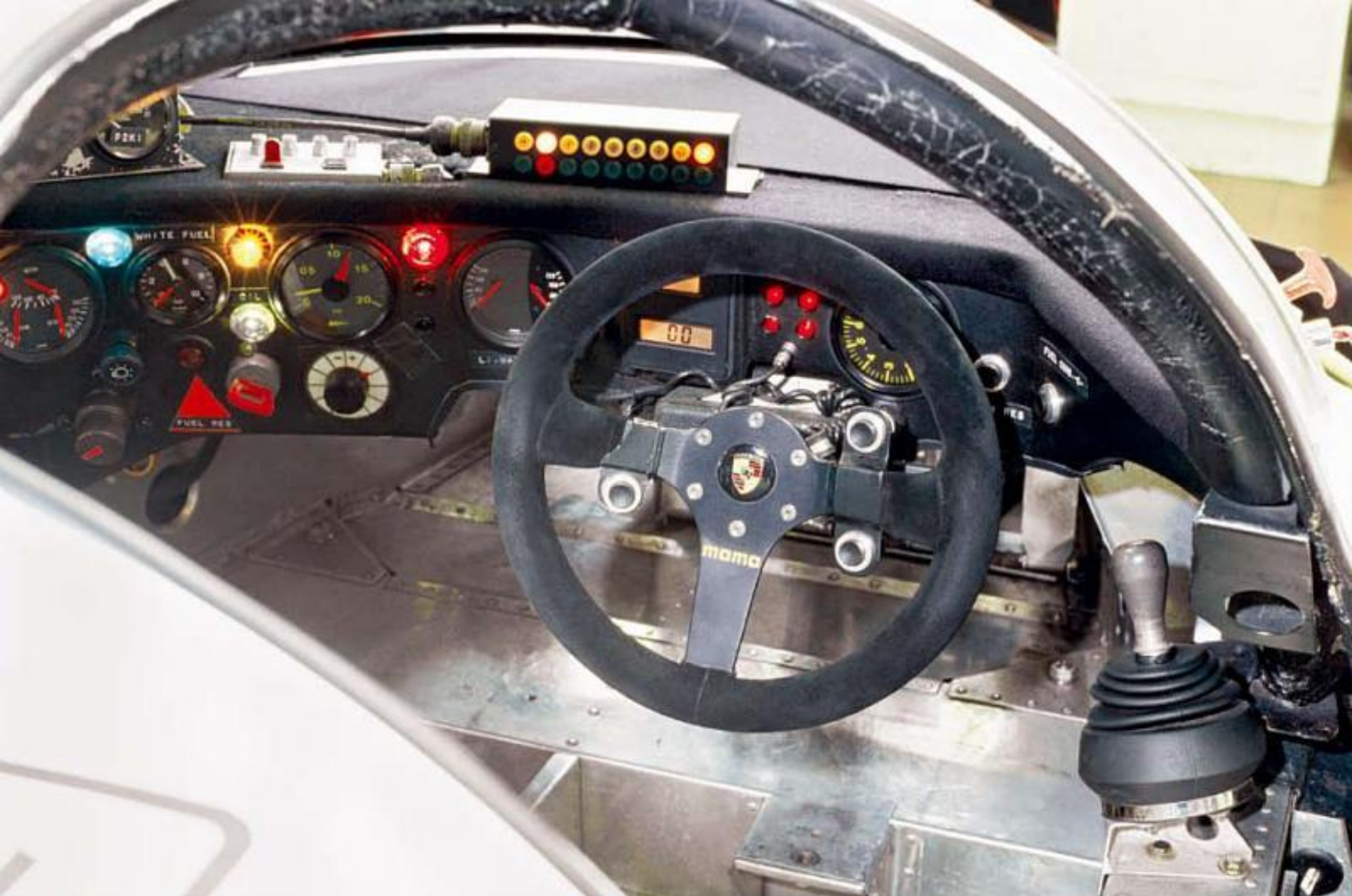
Interior of a works 962C with PDK transmission. Note the selector buttons on the steering wheel, augmenting the traditional shift lever that was moved forward for upshifts and backward for dropping a gear. Electronic controls prevented the driver from over-revving the engine in the heat of competition.
