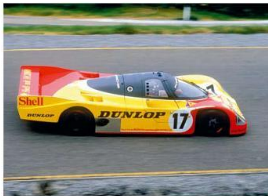
Hans-Joachim Stuck testing the 962.010 at Weissach prior to Le Mans. This is the water-cooled, three-litre car that finished second at the Sarthe, fuel pick-up problems delaying its charge. Note the Shell/Dunlop livery used for 1988.
