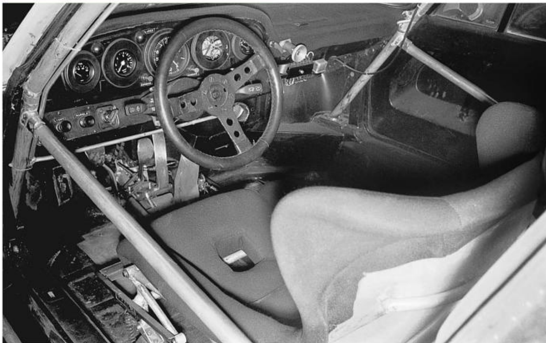
Stripped-out interior of the 935.
