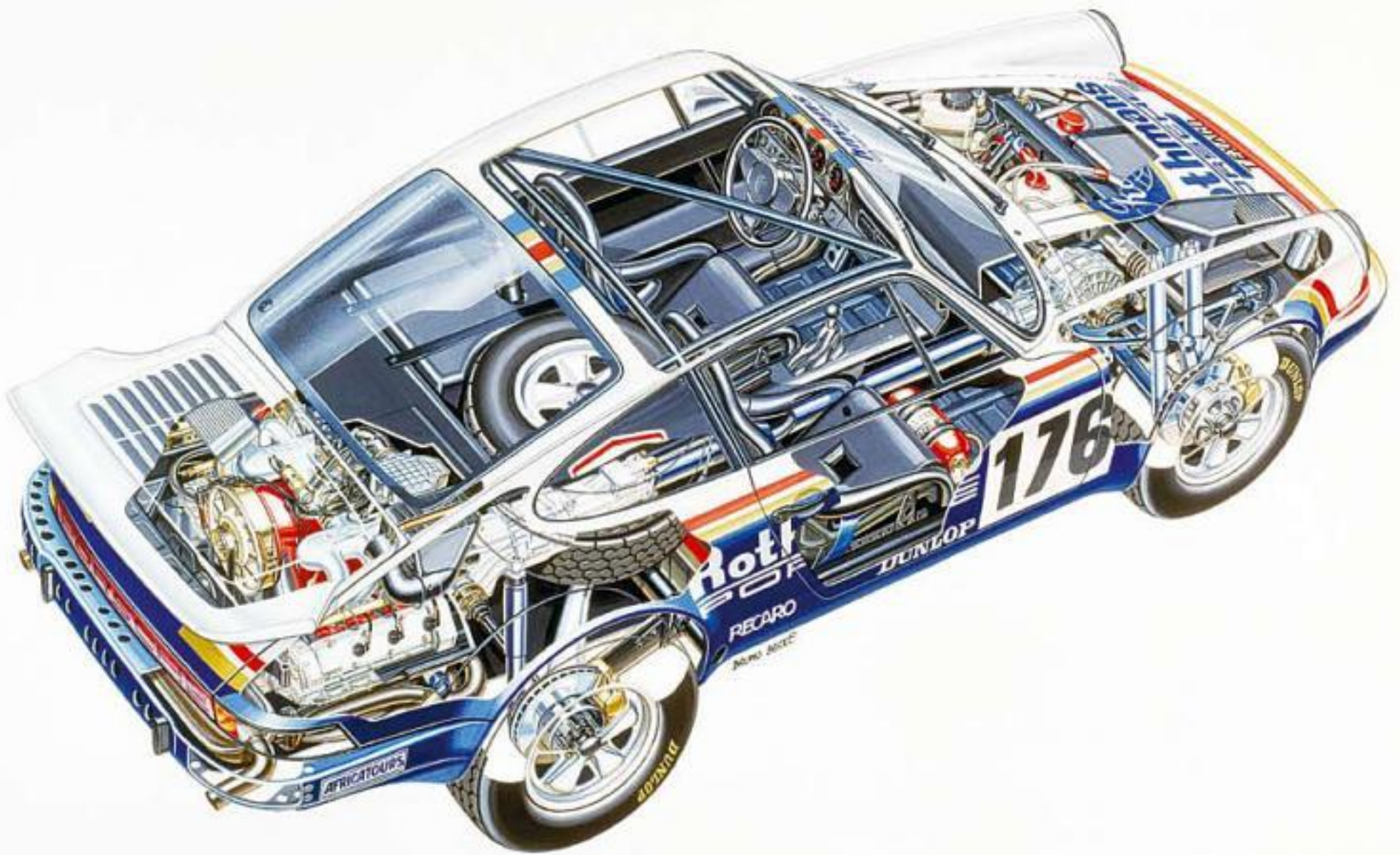
Cutaway drawing of the five-speed Paris-Dakar 911 (Type 953) which tested Porsche's new four-wheel drive system to the limit.
