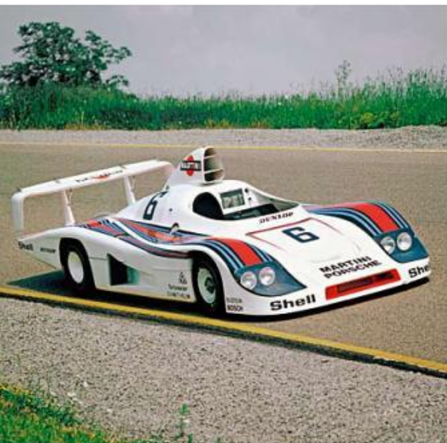
The different tail spoiler and huge NACA duct down the side of the car readily distinguish the 936/78 from its predecessors.
