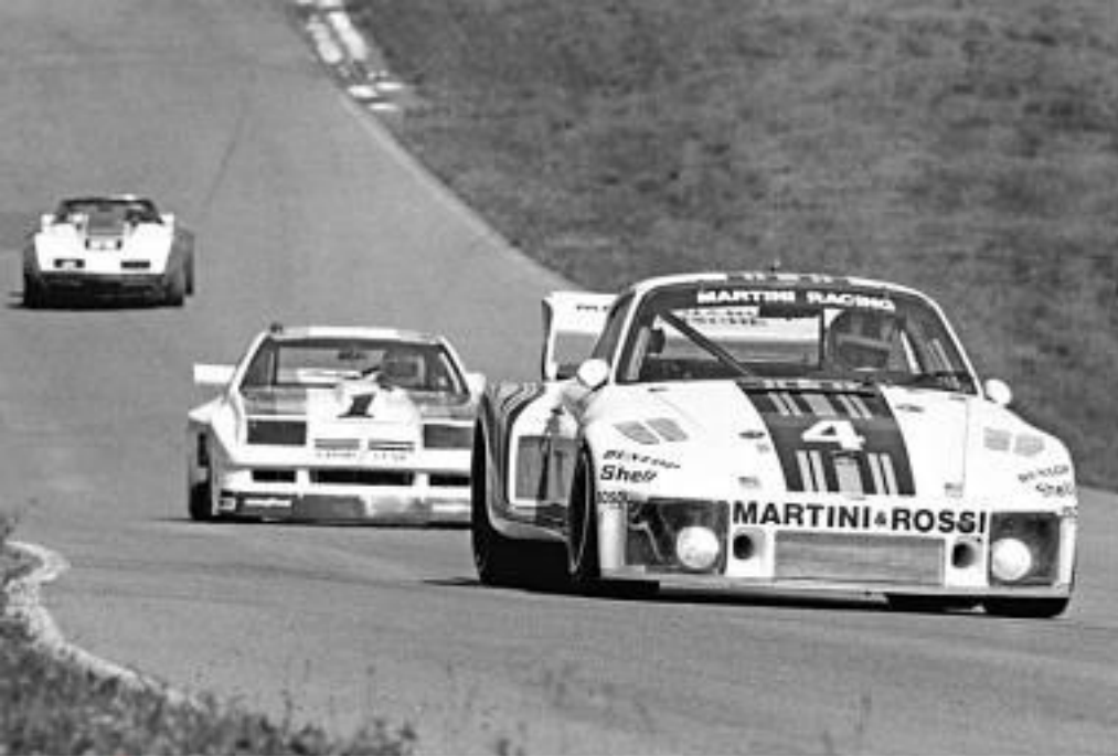
The Stommelen/Schurti 935 at Watkins Glen. Note the wheel covers, fitted halfway through the season to enhance brake cooling.
